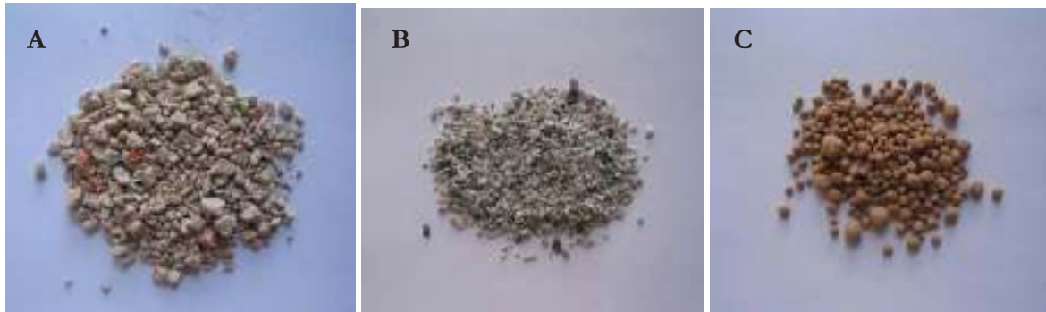
Figure 7. Reactive filter media: Polonite (A), wollastonite tailings (B), Filtra P (C)
